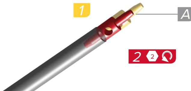
Thread the Reverb Stealth remote hose Barb Connector tool (A) into a 500-700 mm section of shift cable housing, with non-metallic liner, reverse threaded end first. Insert a 2 mm hex wrench through the hole in the tool to rotate it.
