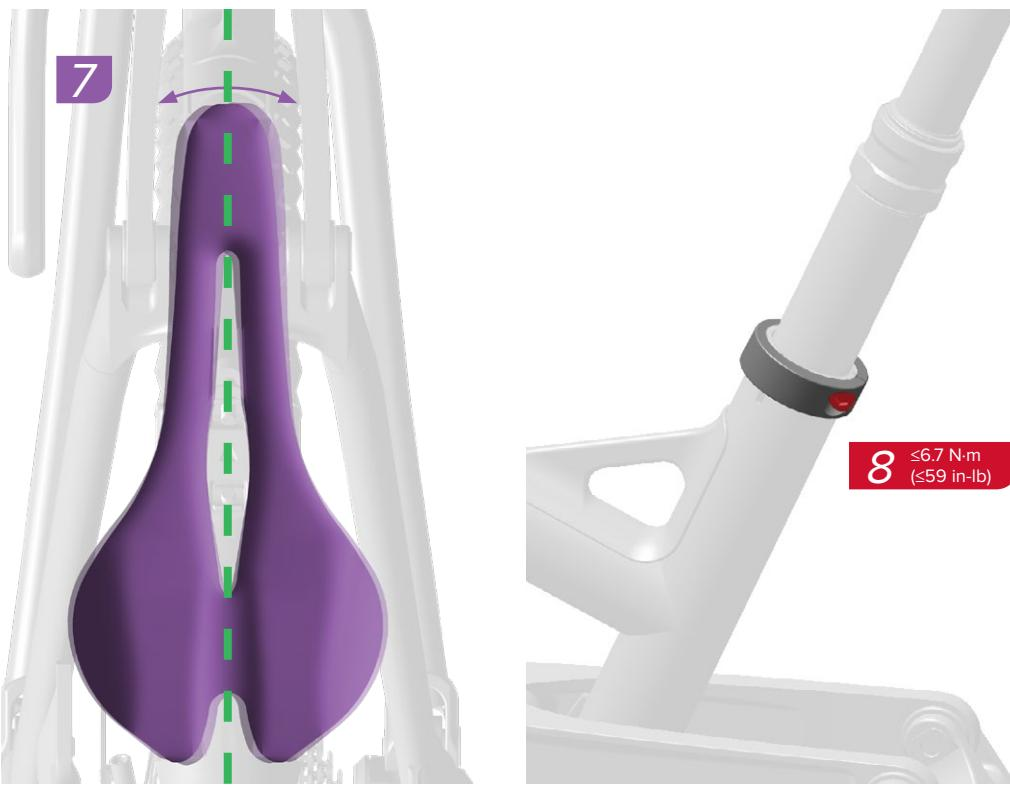
Center the saddle and tighten the seat collar to the frame manufacturer's specification, or  $\leq 6.7 \text{ N}\cdot\text{m}$  ( $\leq 59 \text{ in-lb}$ ), **whichever is lower**.
