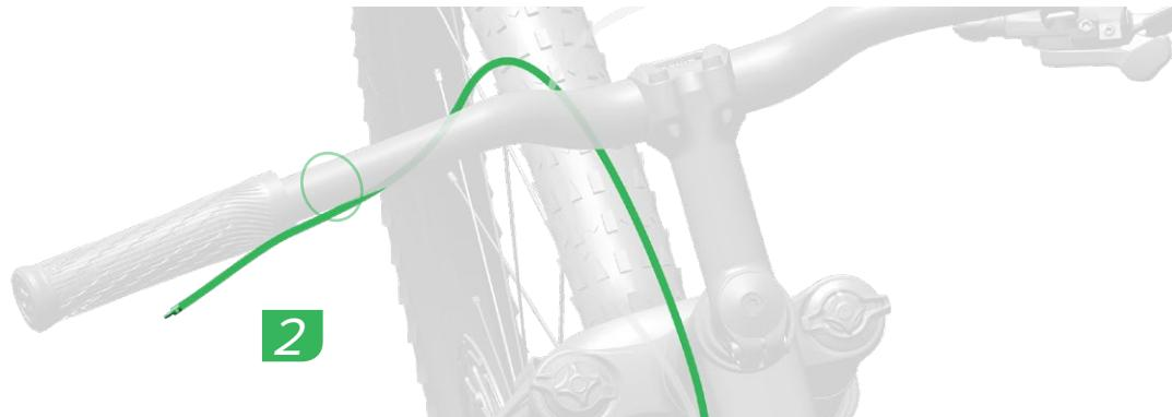
With the seatpost at the preferred ride height in the frame, route the hose to the handlebar remote mount location.
