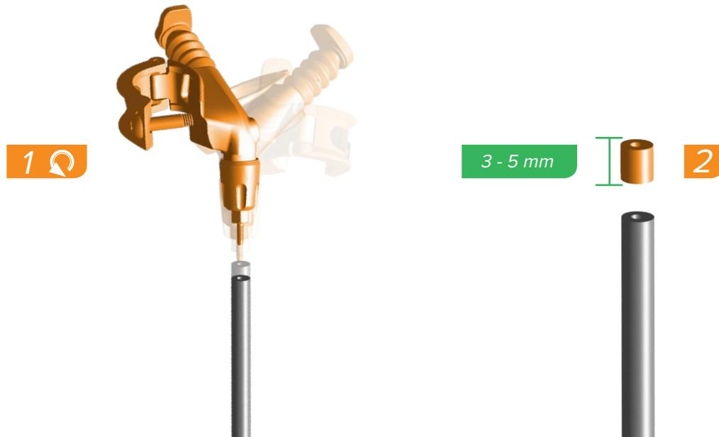
Remove the original remote from the hose and cut 3-5 mm from the end. Cut additional length as needed.
