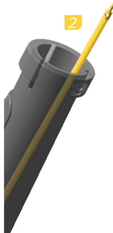
Push the housing into the frame until the Connector tool emerges from the seat tube.
